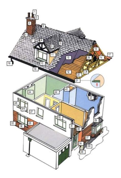
Flashing 4 Ridge ventilation 5 Ridge board Slates/tiles 8 Valley guttering 9 Dormer projection Dormer flashing 10 Dormer cheeks 11 12 Sarking Roof felt 13 Trusses 14 15 Collar 16 Insulation 17 Parapet gutter Eaves guttering 18 Rainwater downpipe 19 20 Verge boards / skews 21 Soffit boards 22 Partition wall Lath / plaster 23 24 Chimney breast
